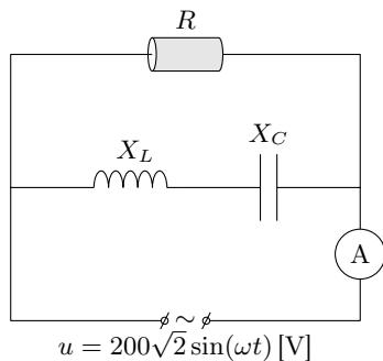
**Zanjirdagi ampermetrning ko'rsatishini (A) aniqlang.**
